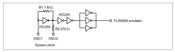
Figure 9 Oscillator Circuit
